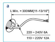
\*For the installation of electrical connections out of sight, a cable leaving the wall no less than 300 mm long with a cable cross-section of 1.5 sq. mm is recommended.
